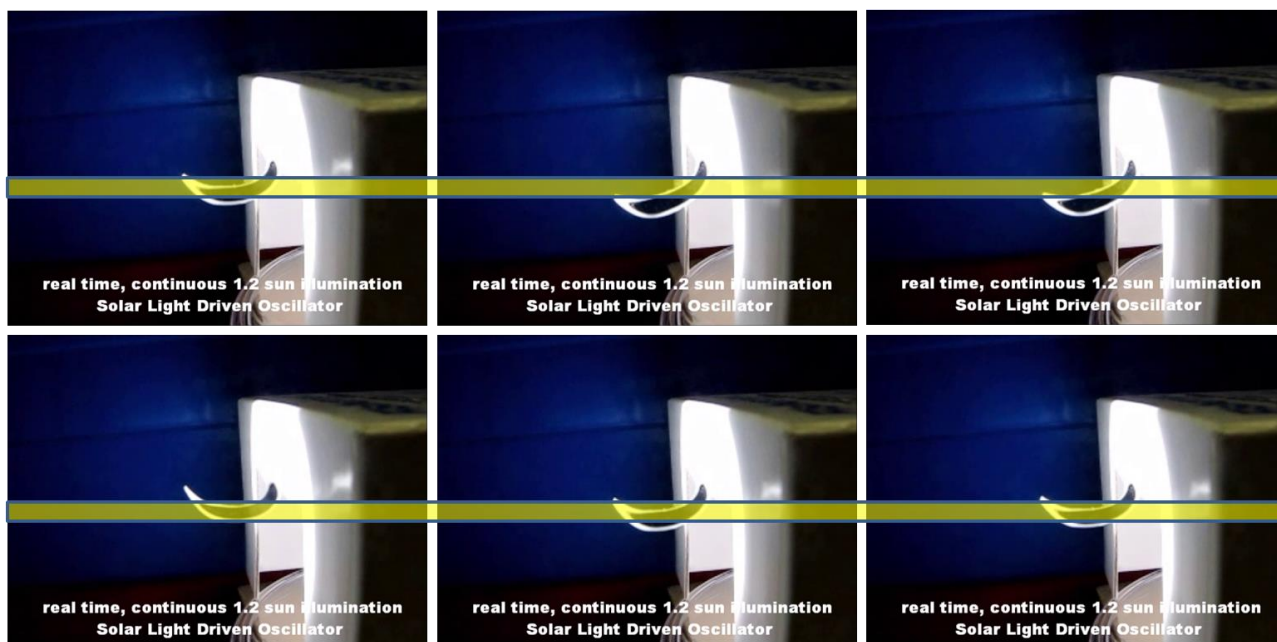
Figure 7: From left to right different frames of the video in Supporting information of X. Zhang et al. [54] regarding the solar light driven oscillator (the horizontal yellow line is added to better highlight the movement of the polymer under illumination).
