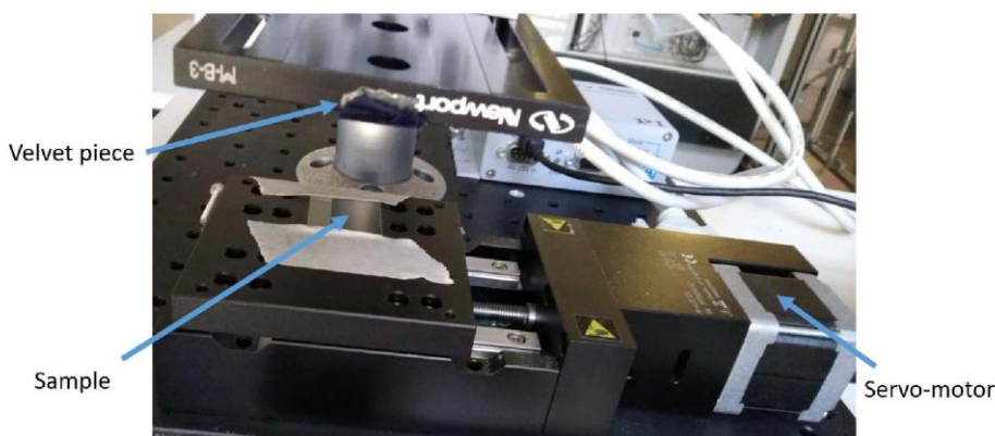
ENEA system used for the rubbing processes before the contact between the slide and the velvet piece.
