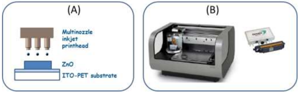
Figure 18. (A) Schema of inkjet process used to produce ZnO seed layer onto ITO/substrate by multinozzle printer shown in (B).
